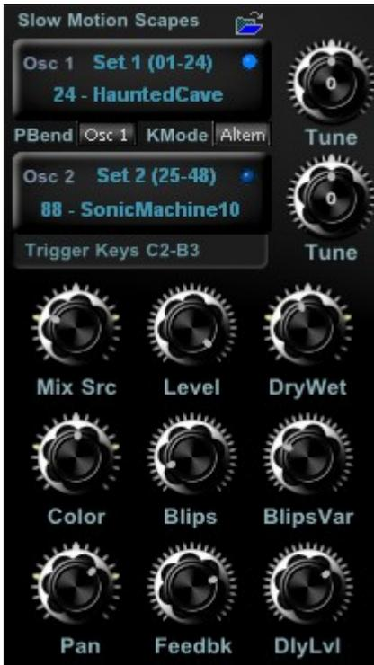
Basically Osc 1 & 2 are triggered alternating, but you can freeze osc. 2 to switch osc 1 only via keytrigger: use button at K(ey)Mode Altrn/Osc 1.
