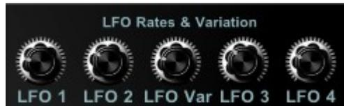
There are four LFO to be contolled in Rate plus a knob to set variation of LFO waves in combination for the four LFO. No LFO is used directly instead there is always used a mix of 2 LFO controlled i.e. mixed by a 3rd LFO to achieve more complex modulation waves giving more longterm variation.
